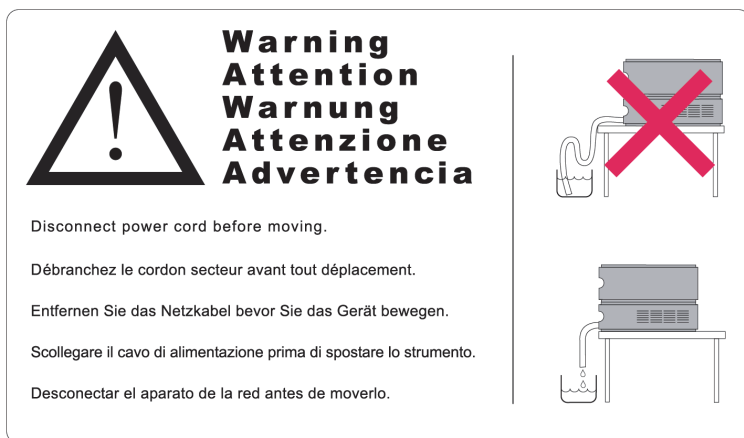
Figure 5 Warning label (illustration for correct waste tubing)
